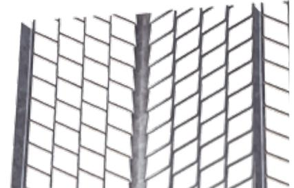
**Quality:** Catnic expanded Rib Lath is manufactured in accordance with BS EN 13658: 2005. Metal Lath - Definitions, Requirements, Test Methods. Part 1 for Internal Plastering. Part 2 for External Plastering. The galvanised steel used in the manufacture of Rib Lath is in accordance with BS EN 10346: 2009 – DX51D+Z275. Where stainless steel is used it is in accordance with BS EN 10088-2-1.4301.
